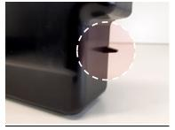
Check if the tab on the backside of the tray is not damaged. In case of damage, please contact the helpdesk of your service provider for a replacement part.
