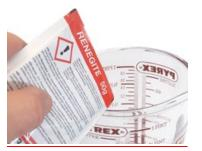
When indicated in the display: it is important to fill the water tank with **500 ml water** in which a descaling agent is fully diluted.
