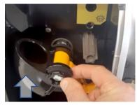
Mount the brewer back in the machine: Slide the brewing chamber back onto the axle.
