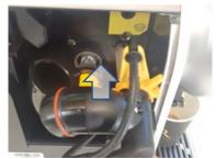
Slide the right part back in, and press slightly until you notice a clicking sound – the brewer is now locked in place.
