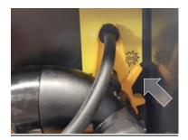
Unlock the brewer: Press the yellow release knob upwards.
