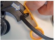
Guide the clip along the edge (on the brewing chamber) as shown here.
