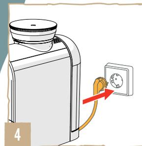
Switch on the Giro by inserting the plug into the socket.
