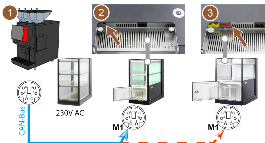
Image: Overview of CAN bus connections from the coffee machine to optional accessories
