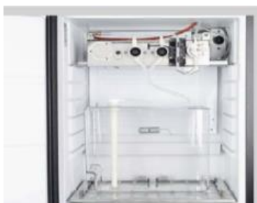
Replenish milk if necessary. Check tray for condensed water and empty if necessary.
