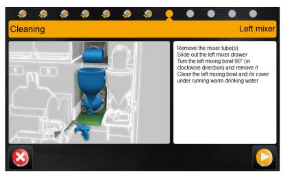
Remove mixer tubes Slide out the mixer drawer and remove the mixer. Clean the bowl.
