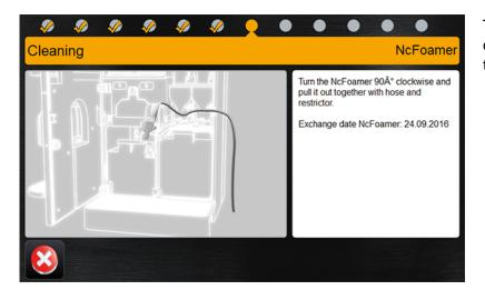
Turn the Ncfoamer 90° clockwise and remove it together with the hose.
