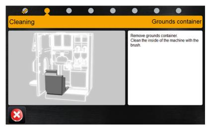
Remove the grounds container and clean the machine inside with a brush.
